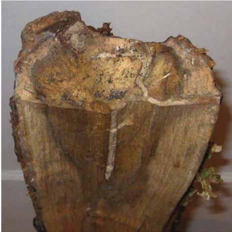
*Notice the concentration of decay at the failure point which is also the location of a spur wound.*
