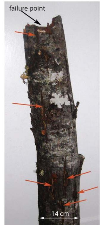
*Orange arrows indicate spur wounds. Notice the proximity of the failure point to the uppermost spur wound.*
